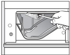
Using a bottle brush remove any detergent or lime deposits from the water inlet valves at the top of the detergent drawer niche.
